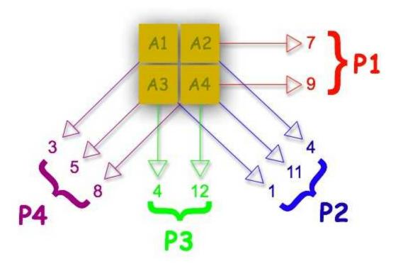
The first projection, P1, is imaged from the right and the second projection, P2, from the right oblique and so on. The projections are firstly added to each as shown below:
