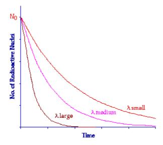
All three curves here are exponential in nature, only the Decay Constant is different. Notice that when the Decay Constant has a low value the curve decreases relatively slowly and when the Decay Constant is large the curve decreases very quickly.
