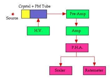
It consists of a scintillation crystal coupled to a photomultiplier tube which is powered by a highvoltage circuit (H.V.). The output voltages are initially amplified by a sensitive pre-amplifier (**Pre-Amp**) as we noted above before being amplified further and conditioned by the amplifier (**Amp**).
