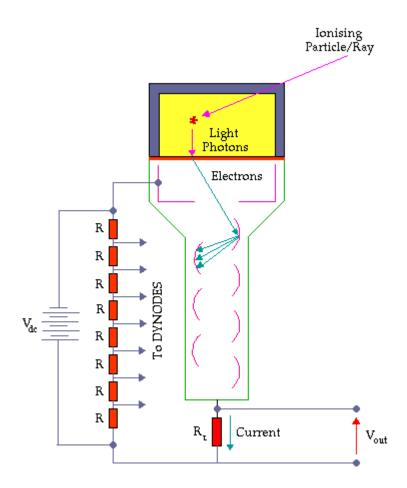
The ionizing radiation produces flashes of light in the scintillation crystal. This light strikes the photocathode and is converted into electrons. The electrons are directed by the grid onto the first dynode.
