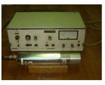
A single channel analyser with a crystal-PMT assembly.
