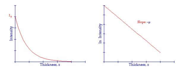
Table 1: Graphical representation of the dependence of radiation intensity on the thickness of absorber: Intensity versus thickness on the left and the natural logarithm of the intensity versus thickness on the right.
