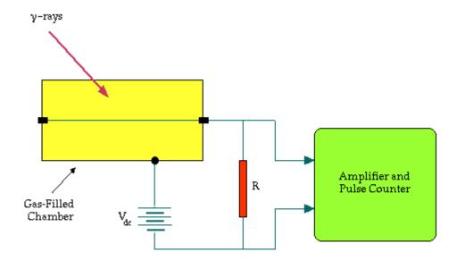
The positive electrode consists of a thin wire running through the centre of the cylinder and the negative electrode consists of the wall of the cylinder. In principle we could make such a detector by getting a section of a metal pipe, mounting a wire through its centre, filling it with an inert gas and sealing the ends of the pipe. Actual detectors are a little bit more complex however but let us not get side-tracked at this stage.
