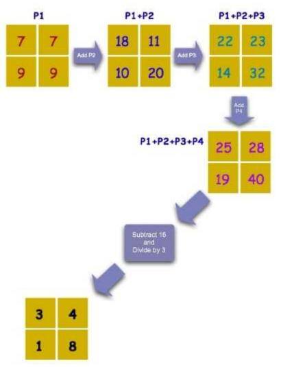
and the summed (or superimposed) projections are normalised to generate an estimate of the radioactivity in each voxel.
