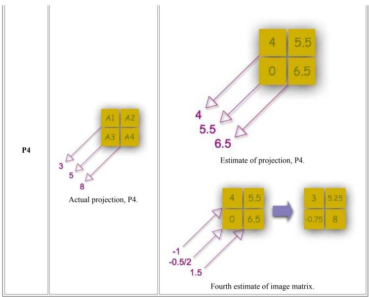
The first estimate of the image matrix is made by distributing the first projection, P1, evenly through an empty pixel matrix. The second projection, P2, is compared to the same projection from the estimated matrix and the difference between actual and estimated projections is added to the estimated matrix. The process is repeated for all other projections.
