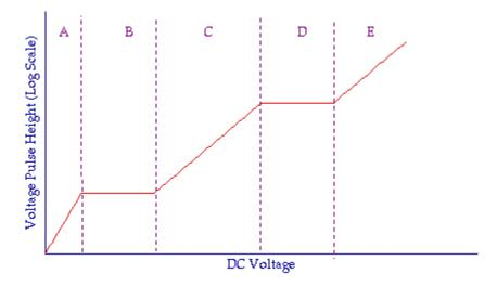
The graph illustrates the dependence of the pulse height on the dc voltage. Note that the vertical axis representing the pulse height is on a logarithmic scale for the sake of compressing a large linear scale onto a reasonably-sized graph.
