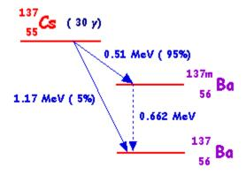
The general method used for decay schemes is illustrated in the diagram below:
