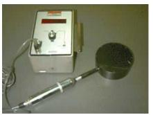
An exposure meter used in radiography.
