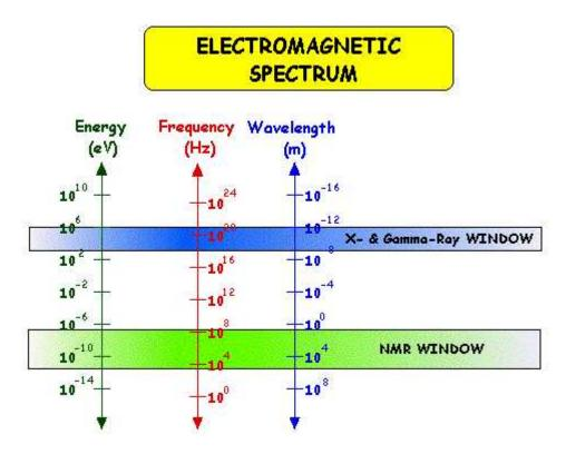
Before proceeding it is useful to pause for a moment to consider the difference between X-rays and gamma-rays. These two forms of radiation are high energy electromagnetic rays and are therefore virtually the same. The difference between them is not **what** they consist of but **where** they come from. In general we can say that if the radiation emerges from a nucleus it is called a gamma-ray and if it emerges from outside the nucleus from the electron cloud for example, it is called an X-ray.
