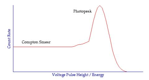
This plot illustrates what is obtained for a monoenergetic gamma-emitting radioisotope, for example <sup>99m</sup>Tc - which, as we have noted before emits a single gamma-ray with an energy of 140 keV.
