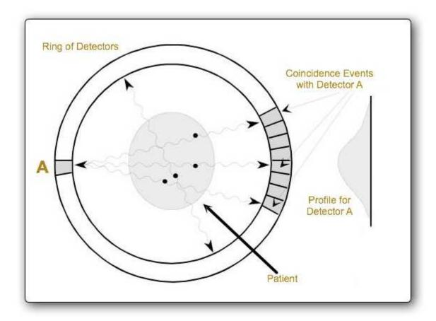
The locations of positron decays within the patient are highlighted by the solid circles in the above diagram. In addition only a few detectors are shown in the diagram for reasons of clarity. Each detector around the ring is operated in coincidence with a bank of opposing detectors and the annihilation gamma-rays thus detected are used to build up a single profile.
