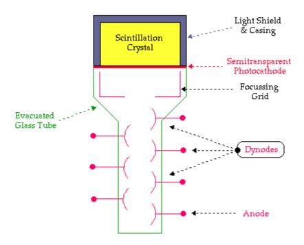
The scintillation crystal, NaI(Tl) is very delicate and this is one of the reasons it is housed in an aluminium casing. The inside wall of the casing is designed so that any light which strikes it is reflected downwards towards the PMT.
