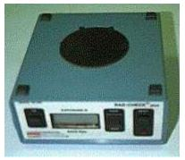
An exposure meter used in radiography.
