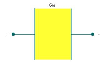
Here we have two electrodes with the gas between them. Something like a capacitor with a gas dielectric.
