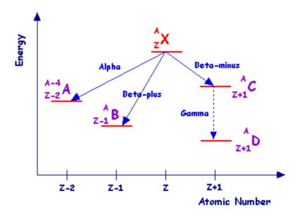
The energy is plotted on the vertical axis and atomic number on the horizontal axis - although these axes are rarely displayed in actual schemes. The isotope from which the scheme originates is displayed at the top - X in the case above. This isotope is referred to as the **parent**. The parent looses energy when it decays and hence the products of the decay referred to as **daughters** are plotted at a lower energy level.
