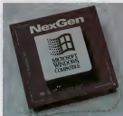
The NexGen Nx586 is one of the first of a new breed of RISC-based processors which can run Intel 80x86 code.
