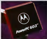
Pippin's CPU will be built around the base-model PowerPC chip, the 603, developed by Apple in conjunction with Motorola and IBM
